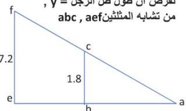
$$\begin{aligned} \frac{1.8}{7.2} &= \frac{y}{x+y} \\ \rightarrow \frac{1}{4} &= \frac{y}{x+y} \\ x+y &= 4y \rightarrow x = 3y \\ \frac{dx}{dt} &= 3 \frac{dy}{dt} \rightarrow \frac{dy}{dt} = \left( \frac{30}{3} \right) \\ \frac{dy}{dt} &= 10 \text{ m/min} \end{aligned}$$
