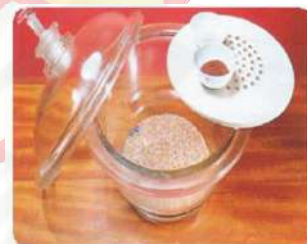
Figure 5 - 7 Silica gel as a desiccant factor
