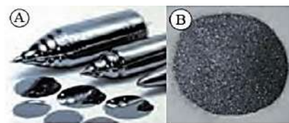
Figure 5-3 Types of silicon A) crystallized B) non-crystallized
